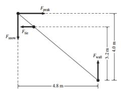
To find the value of  $F_{\text{tie}}$ , you'll need to consider the torques on the rafter. The most convenient choice for a pivot point is the joint where the rafter meets the wall. The sum of the torques around this point is
