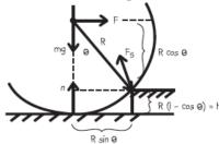
Since you don't know the magnitude or the direction of the step force, you should choose as the pivot point where the wheel meets the step. Before the cart starts moving, the wheel is in static equilibrium, so the sum of the torques around this pivot point should be zero:
